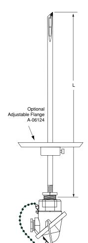
This assembly is particularly suited to measuring temperature of asphalt and other granular materials such as grain, sand, gravel, and pulverized coal. The element is solid 14 gauge with porcelain insulation inside a 1/4" NPT seamless steel case hardened protection pipe. The end of the pipe is cut at an angle to protect the element and allow close contact with the material. The tip of the thermocouple with grounded junction style is welded to the end of the pipe for greater sensitivity.
